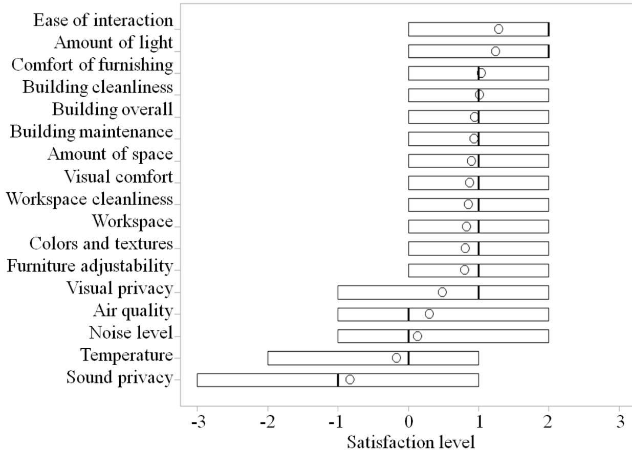
Figure 1. Box plots for satisfaction with parameters assessed in the CBE occupant satisfaction survey. The extremities of the boxes are the 25<sup>th</sup> and 75<sup>th</sup> percentiles. Bold vertical lines indicate median values and dots represent mean values. For all the parameters the minimum and maximum values are equal respectively -3 (very dissatisfied) and 3 (very satisfied).
